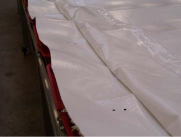
It is advised to start fixing the CARAPAX® roof curtain from the front side of the roof. The roof curtain must be fixed on the first roofstick at both sides with the clamp.
