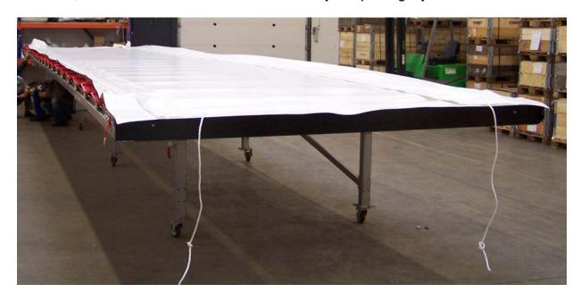
Then the side flaps can be brought down to the sides and fixed with a rivet on the roofsticks.
