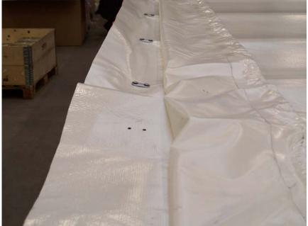
When the CARAPAX® roof curtain is fixed on every roofstick, the first nut can be screwed firmly in place with an air-powered screwdriver. By doing this, the second screw on the clamp will come down so that it becomes easy to put the second nut on it. The second nut can immediately be screwed firmly in place. When this is done, the CARAPAX® roof curtain will already be quite tightly fit on the roof.
